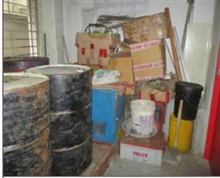
Photo of non-conformity Diesel drums kept with wastage.JPG
